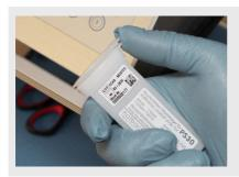
After taking the new shipping container out of the film tubing, it is opened by lifting the cap on one side.
