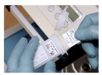
The slide can be easily pulled out of the container after opening.
