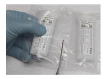
The slides can be separated individually because of the double welding seams in the film tubing.
