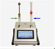
The photo shows the TENAX adapter (green arrow) in operation on the left channel of BiVOC2V2.
