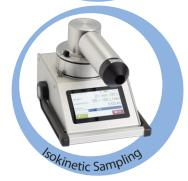
For isokinetic samplings in larger air ducts, the transverse adapter and suitable intake nozzles are available for the air sampling heads LKS 30 and LKS100. It is also possible to load 50 mm PU foam cylinders (without glass fiber pre-filter) for chemical samplings with the transverse adapter.
