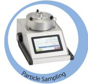
Particle sampling with PS 30 can also capture non-cultivable spores. The evaluation can be done directly after the sampling. This method is ideally suited for remediation inspection. Adhesively coated glass microscope slides are offered as sampling medium. Up to three samplings can be drawn on one slide.
