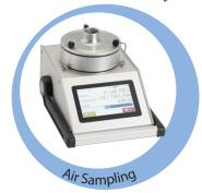
Air samplings on culture media in 83 - 95 mm standard Petri dishes with the air sampling heads LKS 30 and LKS100. A hose connection for samplings from hollow spaces is standard. LKS 30 and LKS100 are validated in accordance with EN ISO 14698-1.
